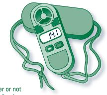
Use a wind-speed gauge to record wind speed and direction before application to decide whether or not the application should proceed and to record wind speeds at various intervals during the application
